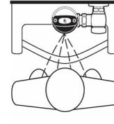
2. As the user enters the beam's effective range (15" to 30") the beam is reflected into the Scanner Window and transformed into a low voltage electrical circuit.
