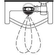
3. When the user steps away from the Sensor, the Sensor initiates an electrical signal that operates the Solenoid. This initiates the flushing cycle to flush the fixture. The Circuit then automatically resets and is ready for the next user.
